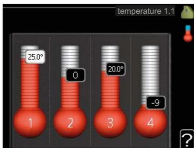
The value in the display appears as a temperature in °C if the heating system is controlled by a room sensor.
