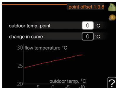
Select a change in the heating curve at a certain outdoor temperature here. One step is usually enough to change the room temperature by one degree, but in some cases several steps may be required.
