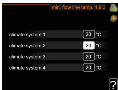
Set the minimum temperature on the supply temperature to the climate system. This means that VVM 500 never calculates a temperature lower than that set here.
