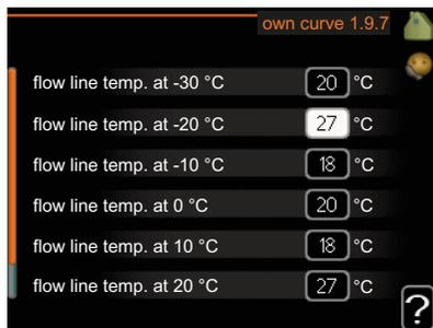
You can create your own heating curve here, if there are special requirements, by setting the desired supply temperatures for different outdoor temperatures.
