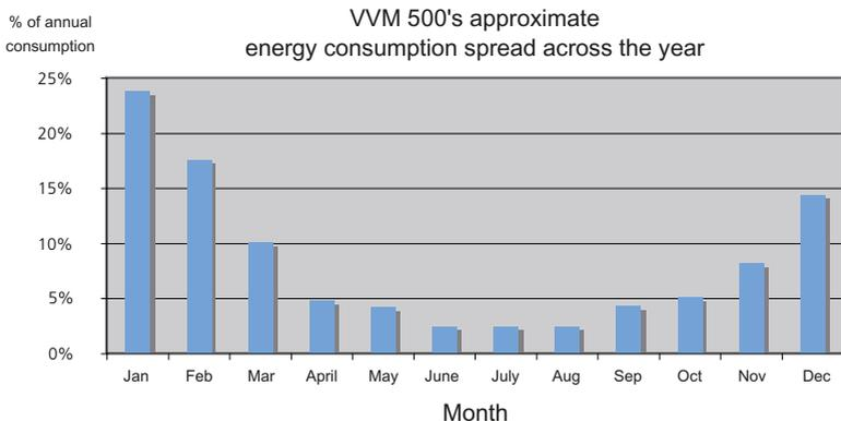
Increasing the indoor temperature one degree increases the energy consumption by approx. 5%.
