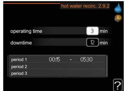
Set the hot water circulation for up to three periods per day here. During the set periods the hot water circulation pump will run according to the settings above.
