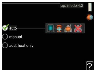
The indoor module operating mode is usually set to "auto". It is also possible to set the indoor module to "add. heat only", but only when an addition is used, or "manual" the select yourself what functions are to be permitted.
