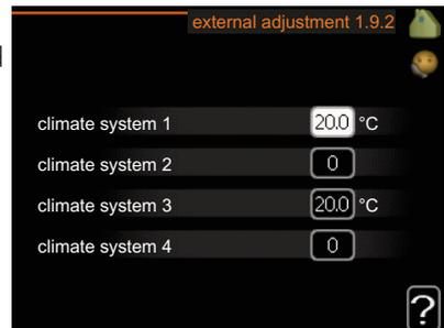
Connecting an external contact, for example, a room thermostat or a timer allows you to temporarily or periodically raise or lower the room temperature. When the contact is on, the heat curve offset is changed by the number of steps selected in the menu. If a room sensor is installed and activated the desired room temperature (°C) is set.
