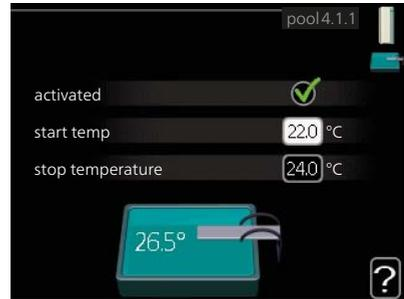
Select whether the pool control is to be activated and within what temperatures (start and stop temperature) pool heating must occur.
