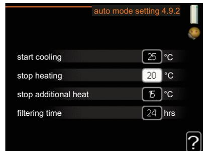
When the operating mode is set to "auto", the indoor module selects when start and stop of additional heat and heat production is permitted, dependent on the average outdoor temperature. If accessories for cooling are present or if the heat pump has the integrated cooling function and it is activated in the menu you can also select the start temperature for cooling.
