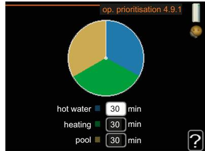
Choose here how long the installation should work with each requirement if there are several requirements at the same time. If there is only one requirement the installation only works with that requirement.
