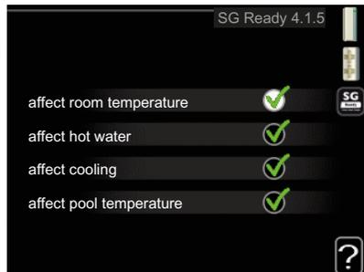
With low price mode of "SG Ready" the parallel offset of the indoor temperature is increased by "+1". If a room sensor is installed and activated, the desired room temperature increases by 1 °C.
