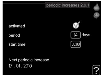
To prevent bacterial growth in the water heater, the heat pump and any additional heat can increase the hot water temperature for a short time at regular intervals.
